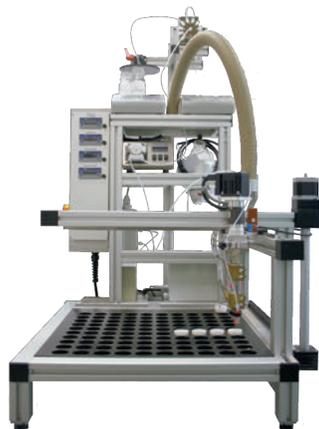
Liquids, solids and melts can be filled into vessels with the formulation and filling system featuring freely programmable mixing ratios.
