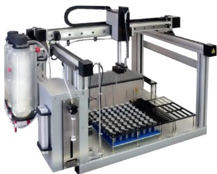
Our synthesis robots offer a similar range of functions such as for the automation of complete synthesis chains, including the fully automatic preparation of slides for microscopic analysis.
