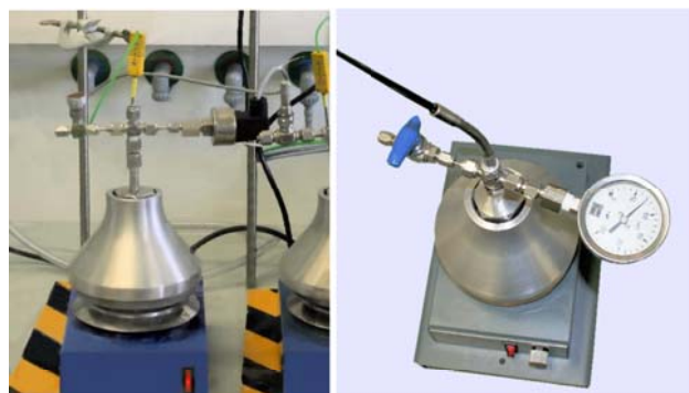
Pressure Reactor 20 ml, heated and agitated with Magnetic Stirrer; on the right: Reactor with fibre-optic ATR Sensor
