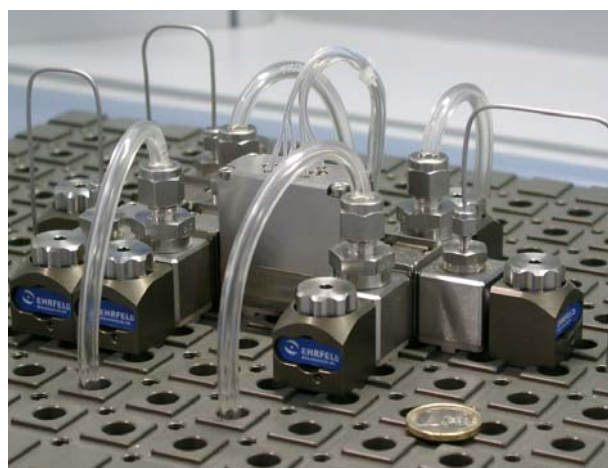
Modular Micro-reaction System: Example for a single stage synthesis for heterogeneous conversions at solid catalysts
