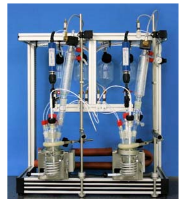
Parallel reactor system with 2 reactors and MultiLab tempering system.
