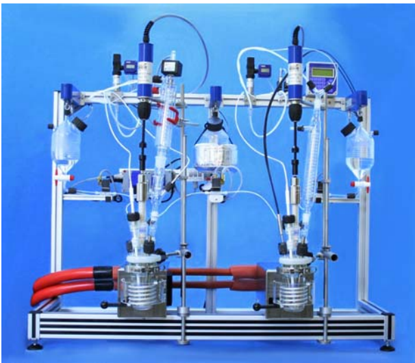
Custom-made Parallel Reactor System for crystallisation screening with turbidity sensor. Joint heated dosing vessel.
