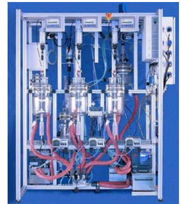
Threefold parallel reactor system with 2 l reactors, parallel, selective dosing from the receiver tanks a, b and p.
