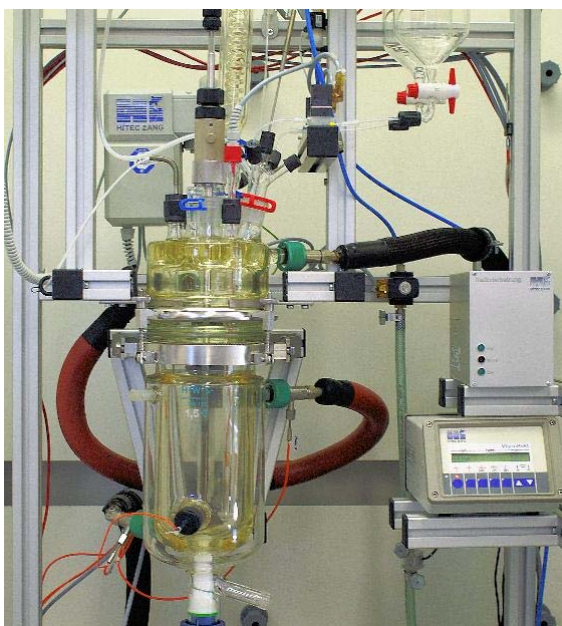
Customer specific reaction calorimeter with heated cover and front side special nozzle.
