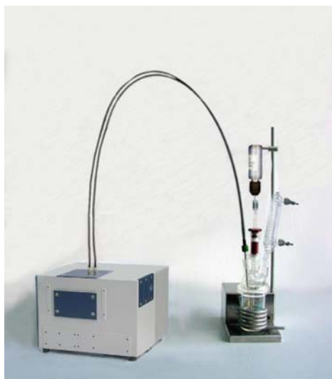
MoleculeEye ATR-probe in a MultiLab 250 ml reactor
