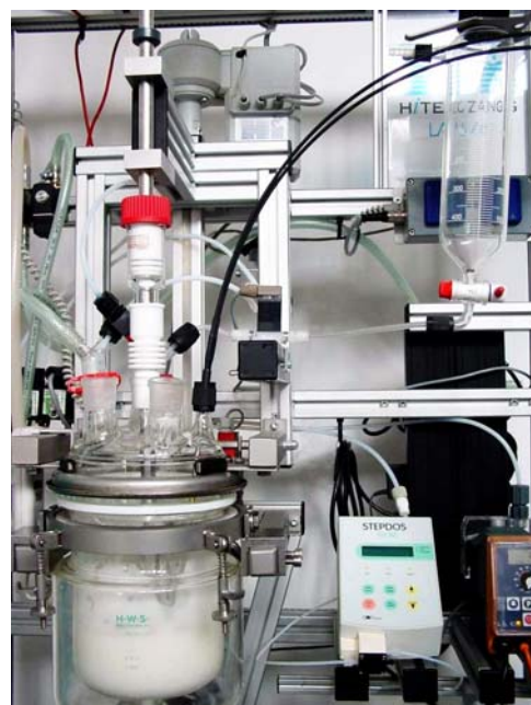
MoleculeEye ATR Probe mounted in a 2 litres LabKit Reaction Plant
