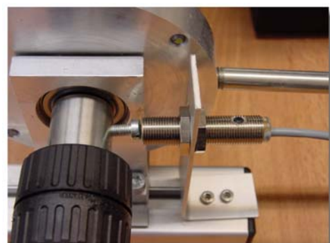
Inductive Proximity Switch as a Rotational Speed Sensor
