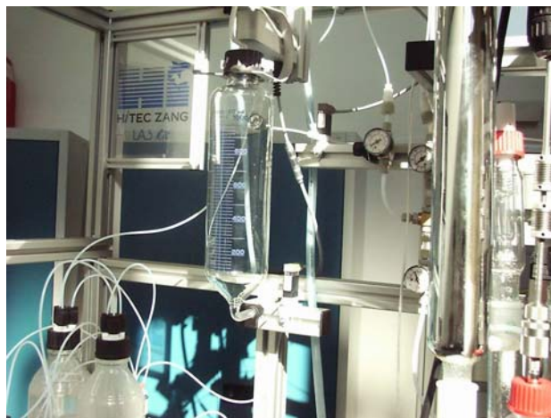
Distillate weighing and separate bottling of the fractions: on the left: collection vessels, center: GraviDos distillate scales, right: rectification column
